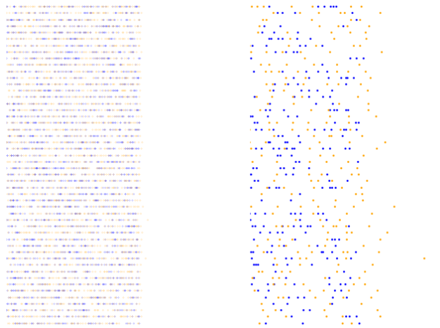
Figure 4: Raster plots of a 50 neurons network, with \lambda = 6.7 , \beta = 10 and \theta = 5 . Left, from time 0 to 14; right from time 12 to 14. Dots are blue when the synapse is facilitated and orange otherwise
